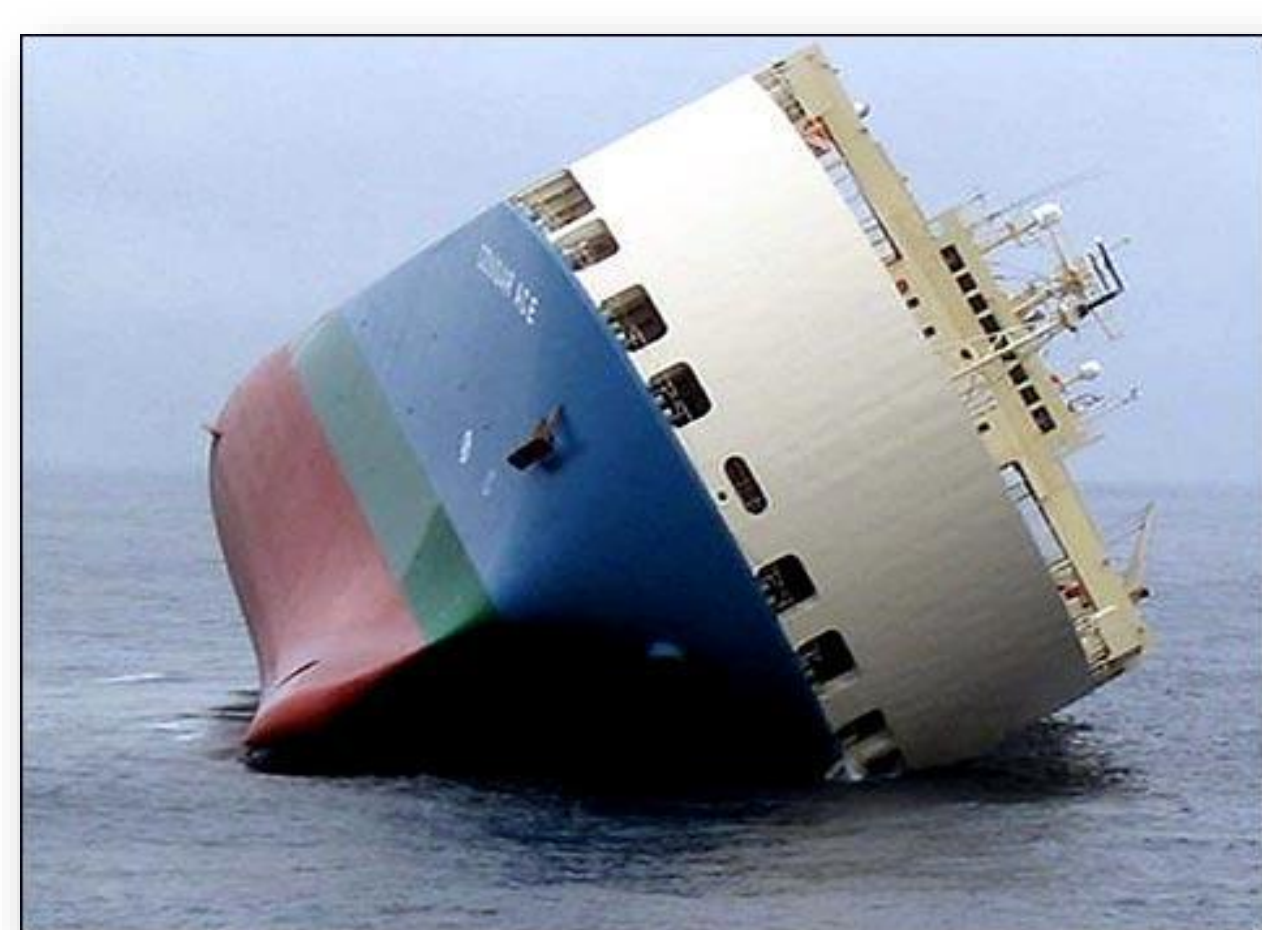
Ship listing due to shifting liquid payload
