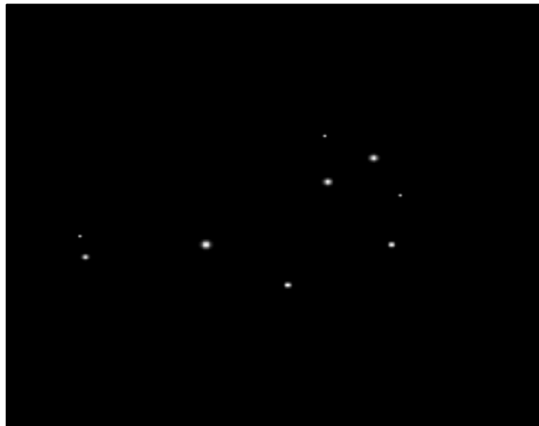
Fig. 60. The estimated image of the Pleiades resulting from the Gaussian phase retrieval algorithm applied to the spectrum shown in Fig. 59. The continuous image is point sampled for display.
