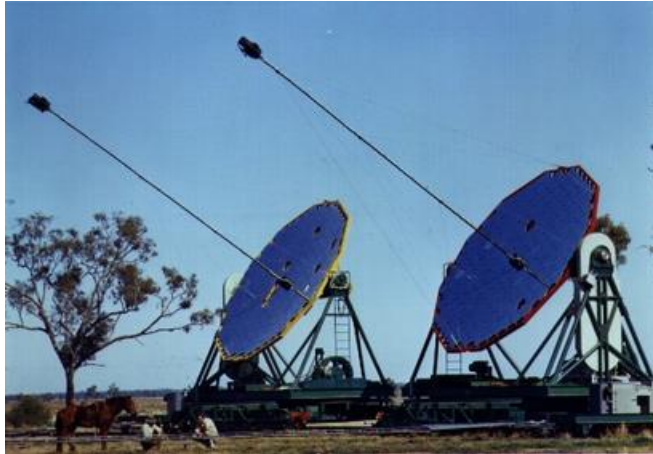
Fig. 12. Photograph of the Narrabri stellar interferometer used by Hanbury Brown and Twiss [24].
