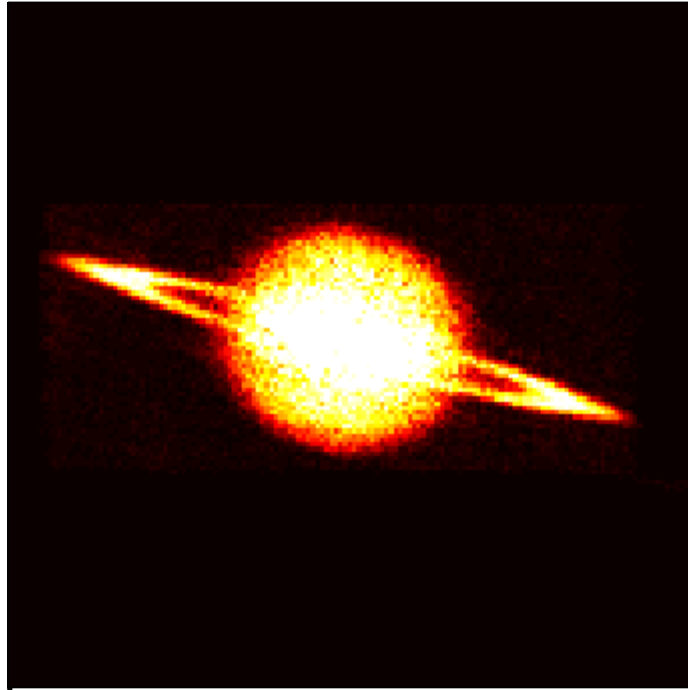
Fig. 34. The result of the image averaging algorithm using twenty image estimates with a Fourier modulus SNR of 0.48.
