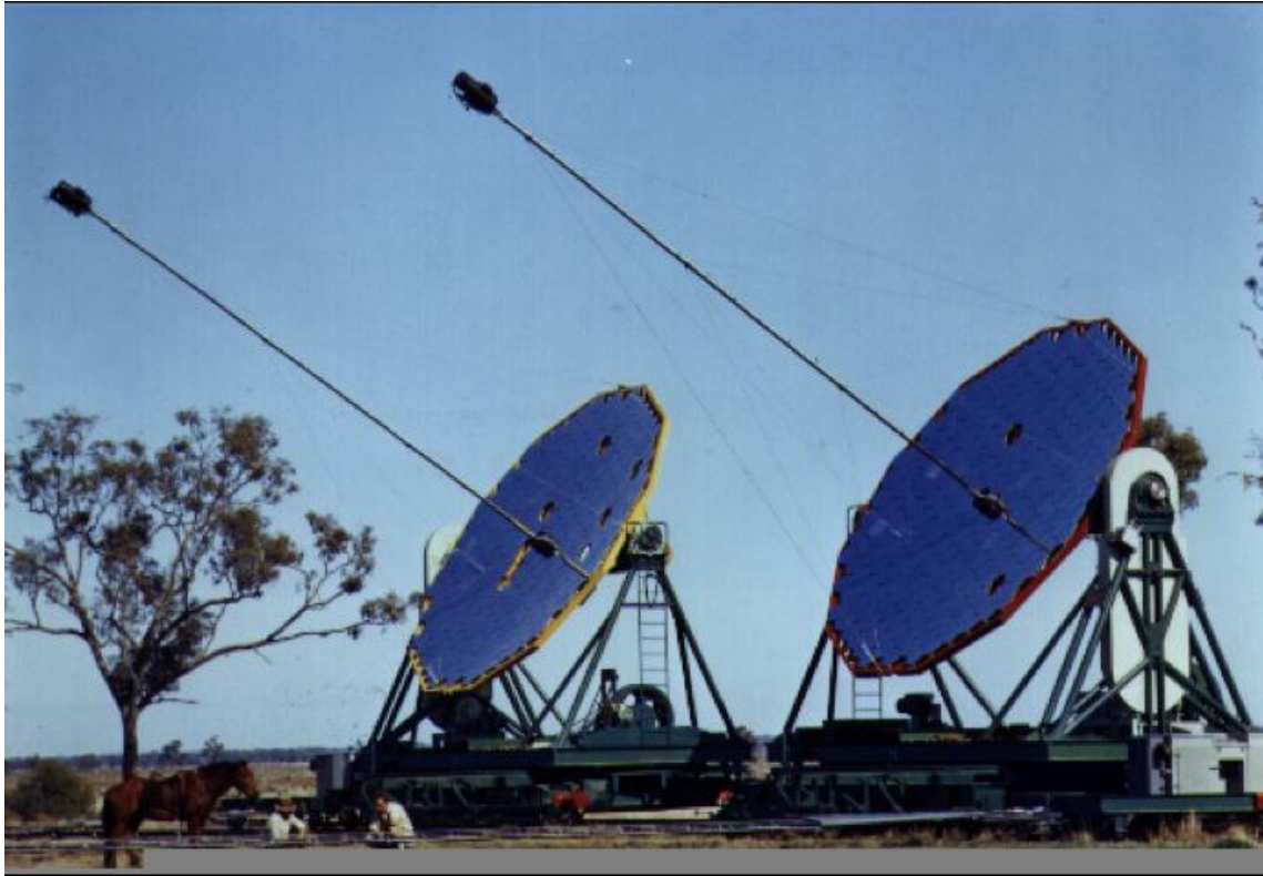
Fig. 10. The Hanbury Brown-Twiss interferometer at the Narrabri observatory. Shown are the two light collectors with photodiodes located on the center mast. The two apertures are on a circular track allowing freedom of baseline and orientation.
