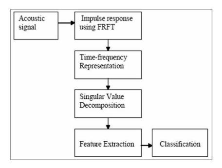
Figure 1. Block diagram of the proposed technique.
